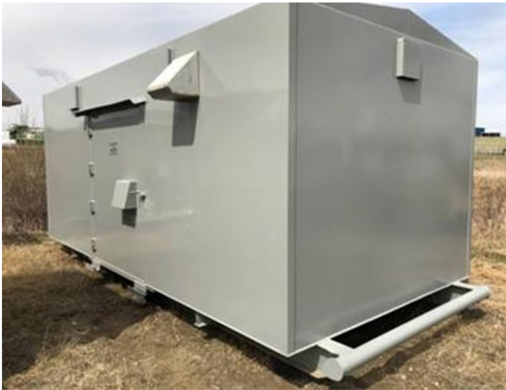
Figure 1.18-9: Example of explosive magazine that will be used for the Tenas Project
