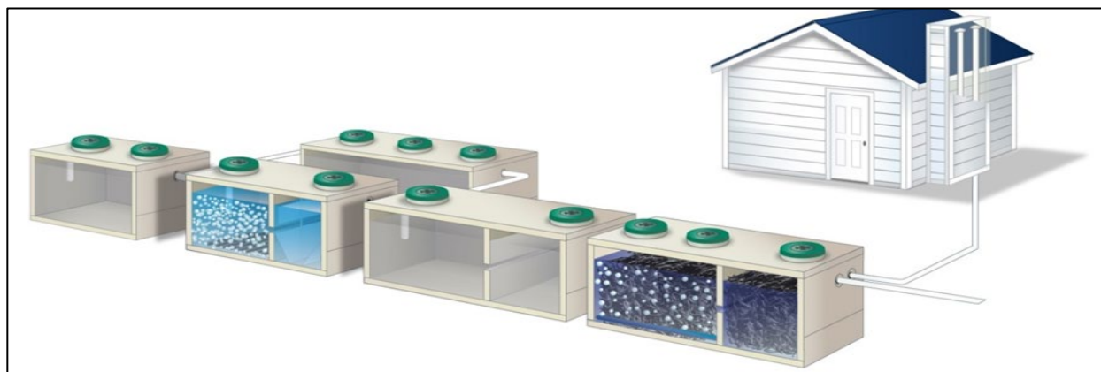
Figure 1.17-5: Example of a Sewage Treatment Plant
