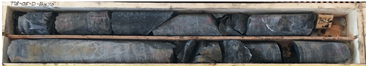
Figure 1.13-5: Core picture of mudstone rock type
