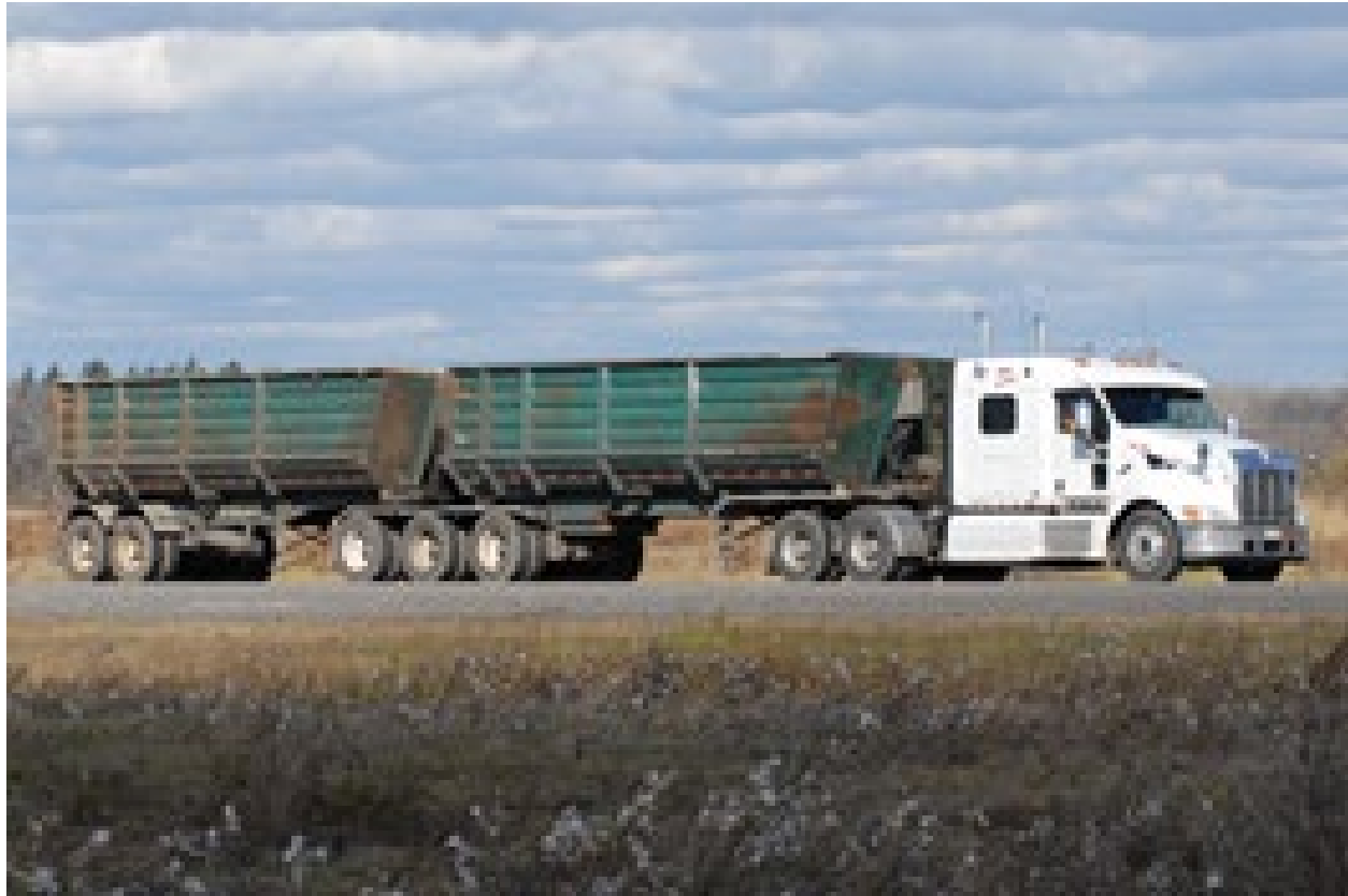
Figure 1.15-13: Super B-train truck configuration
