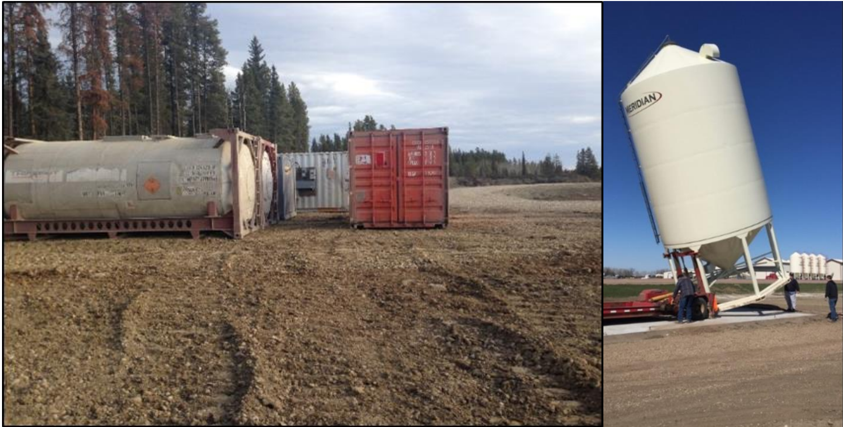
Figure 6.3-2: Photo of 1 x 30 tonne Emulsion Silos for storage and 1 x 50 tonne ammonium nitrate fuel oil (ANFO) silo
