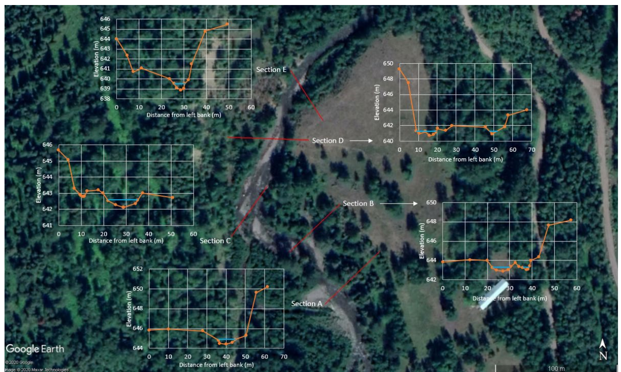
Figure 2-4: Surveyed cross sections near the Goathorn Creek discharge point
