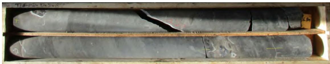
Figure 7-4: Example Core of Sandstone Rock Type
