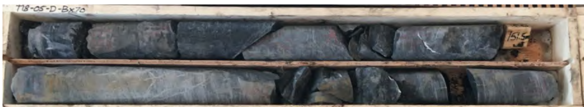
Figure 7-2: Example Core of Mudstone Rock Type
