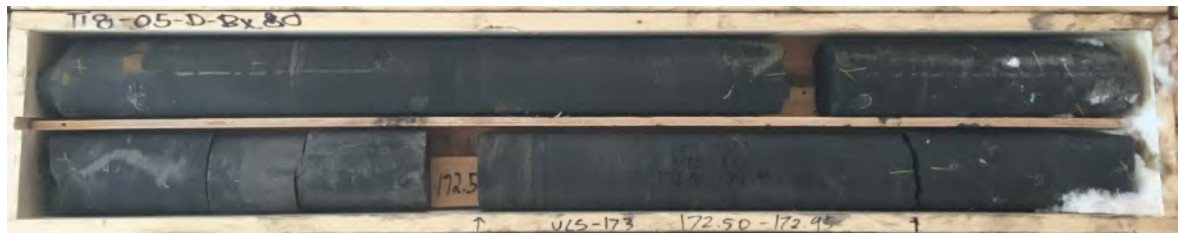
Figure 7-3: Example Core of Siltstone Rock Type
