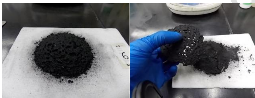
Figure 1: Stockpile treated with 829C (left). Patchy crust lifted off stockpile (right) To compare the two crust compositions: 829C Crust Video And ET Crust Video
