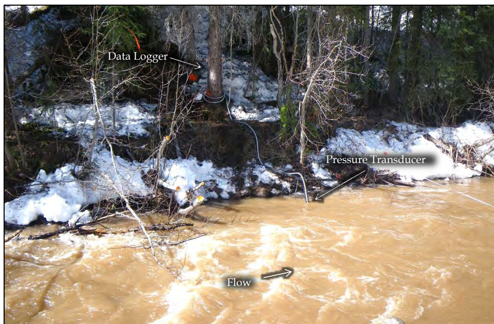
Photo 7.4-2. Hydrometric monitoring station Tenas-Hydro B. May 2, 2018.
