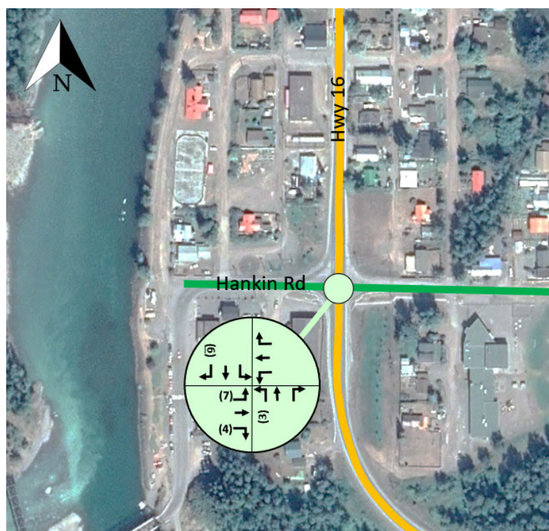
Figure 7: Possible PM Peak Hour Trips Generated by the Tenas Mine (background traffic removed)
