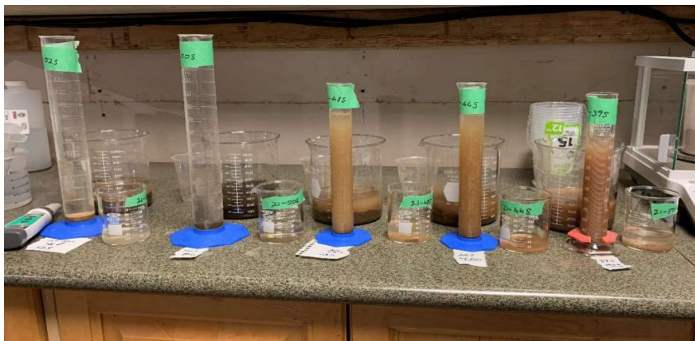
Figure 2: Settlement with Chemical Addition & Filtration
