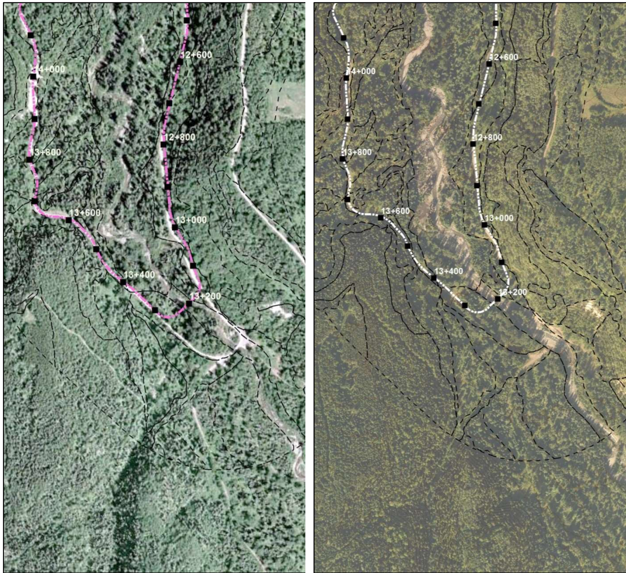
Figure 2-12: Goathorn Creek near the proposed bridge site in 2006 (left image) and 2017 (right image). Note the channel widening following the flood in June 2013.
